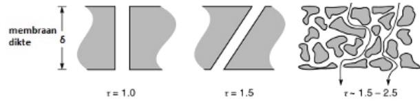
Figuur 1: Cross-sections of porous membranes with different tortuosities (2004) door R.W. Baker
