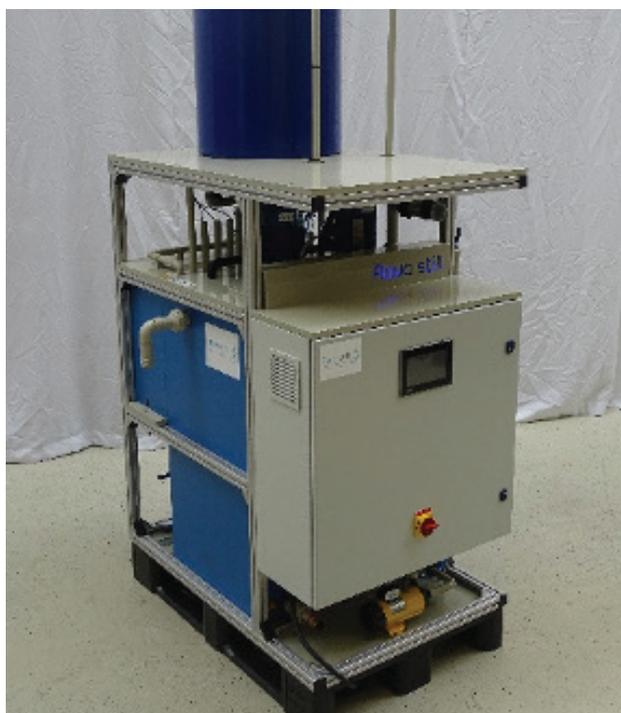
A small MD pilot with a full size module and a total membrane area of 26m<sup>2</sup> was integrated within a waste water stream inside a dye producing factory. Cooling water was taken from a pond and heat was electrically generated because of scale.
